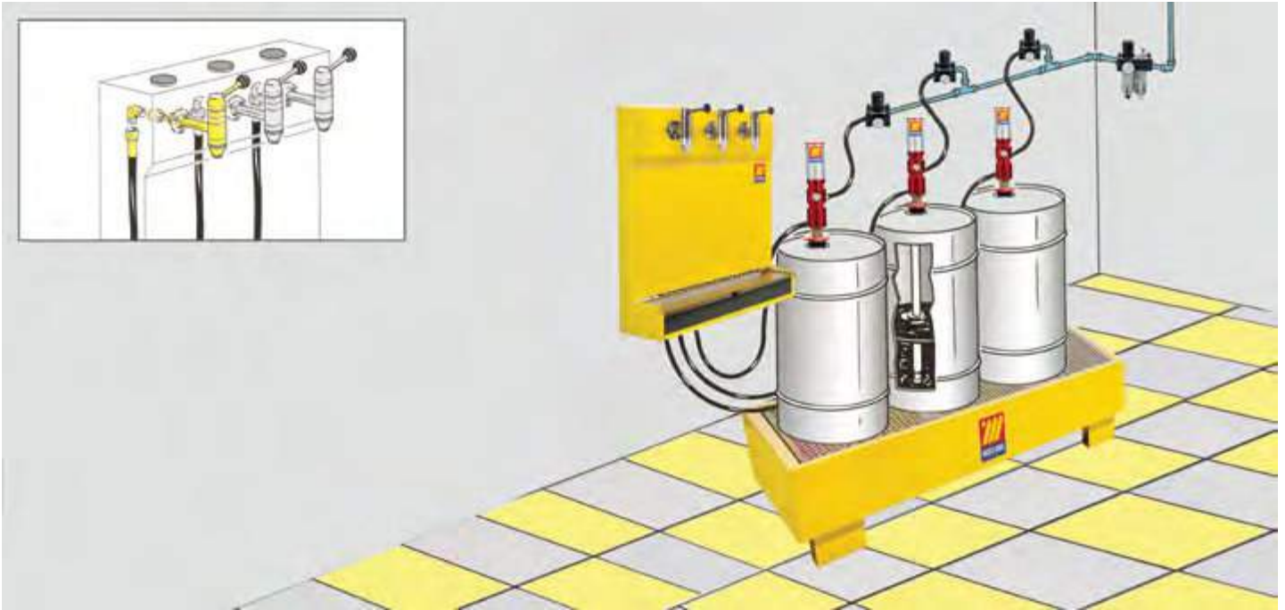
Example of installation with flexible hose
