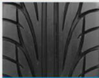
The Unidirectional tire main feature is the "arrow" shaped pattern. All grooves point in the same direction, increasing water dispersion braking performance. For high-speed performance.
