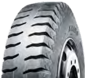
LL159 Bias Truck/Bus Tire 1.Available for heavy load. 2.Good wear resistance. 3.Stable performance.
