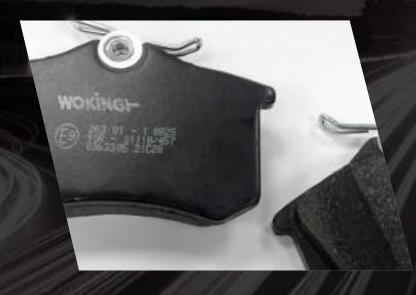
ECE R-90 covers the performance, mechanical characteristics, packaging and production of all brake pads manufactured in Europe effective from 31 March 2001
