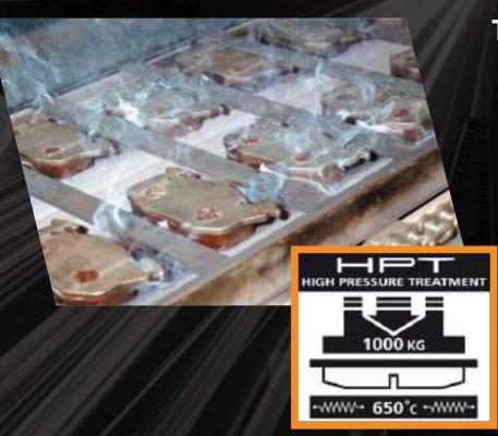
This process provides a shorter bedding-in period and an efficient brake operation just upon installation as typical O.E.M.:
